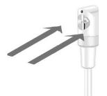
The correct measuring value is determined by rotating the probe slightly in both directions until the maximum value is displayed.
