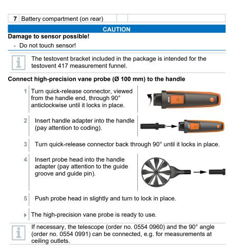
3.5 Vane probe (Ø 100 mm) with Bluetooth<sup>®</sup>, including temperature sensor (0635 9431)
