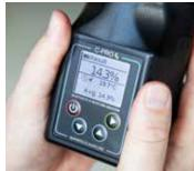
Press the test button and read the moisture content directly from the display.
