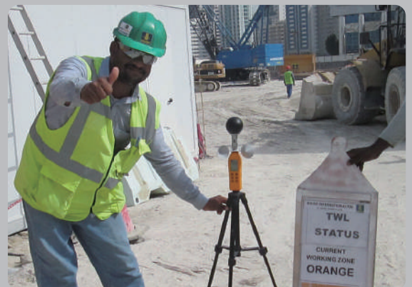
TWL-1S utilized for heat risk assessment at worksite in Abu Dhabi.
